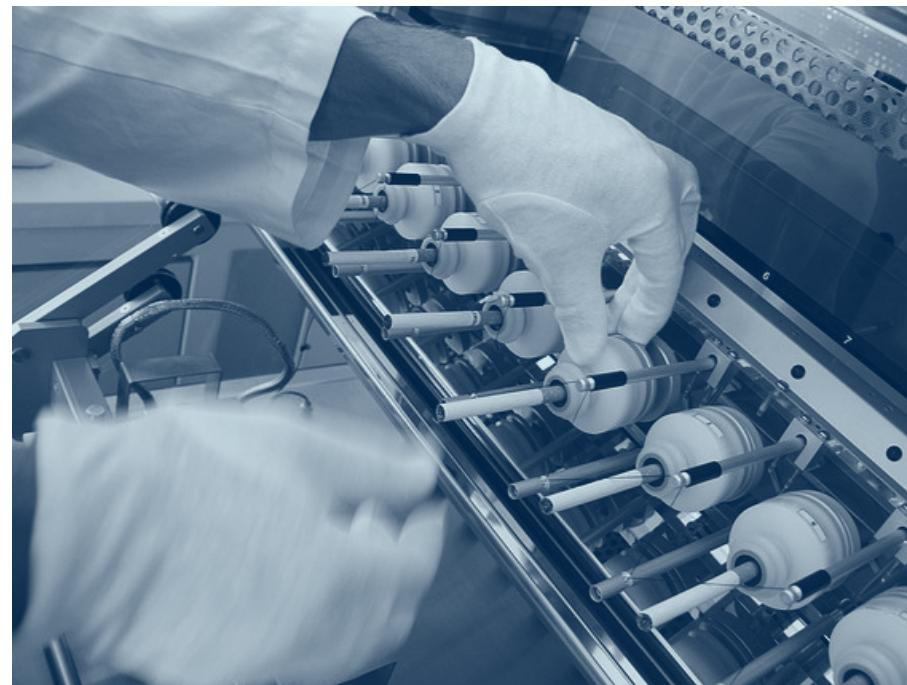
A smoking machine (see picture) is used to test emissions in cigarette smoke as a part of the International Organization for Standardization (ISO) method. Under the ISO method, the machine smokes a cigarette with a 2 second puff of 35 ml every 60 seconds.
